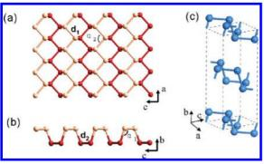
**Figure 1.** (a) and (b) Projections of a single layer BP on the *ac* and *bc* plane. The upper and lower atoms are presented in pink and red, respectively. (c) Schematic illustration of unit cell, showing a shift of *a*/2 units between adjacent layers.
