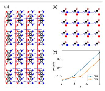
FIG. 2. (a) A chimera lattice with  $4 \times 4$  unit cells. Dots represent Ising spins and lines indicate couplings. (b) Tensor network representation, where each node has a degree of freedom of four spins. (c) Wall clock time for computing the ground state energy of Ising spin glass on the chimera graph with the  $L \times L$  unit cell ( $8L^2$  spins).
