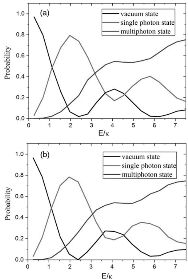
Fig. 5. Probabilities of different photon states versus driving pulse with different wave shapes: (a) sine shape and (b) rectangular shape.
